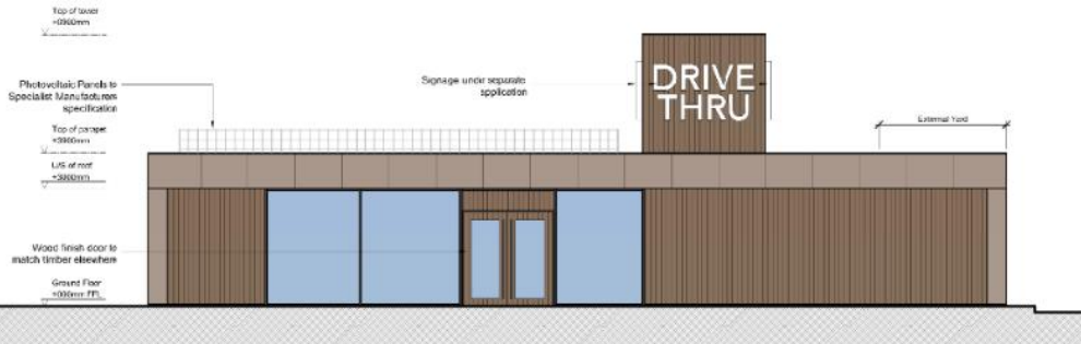
South West (Main Entrance) Elevation Scale 1:100
